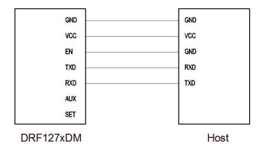
Figure 6: Pin Connection in Configuring the Module
