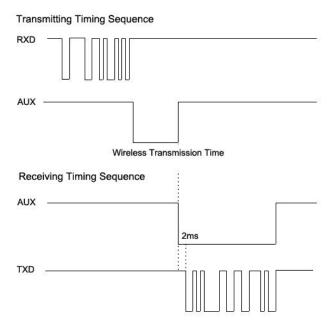
Figure 2: DRF1276DM Timing Sequence
