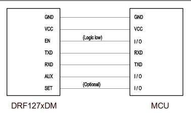
Figure 1: Pin Connections in Standard Mode
