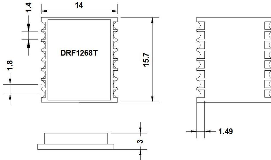
**Figure 3: Mechanical Dimension**
