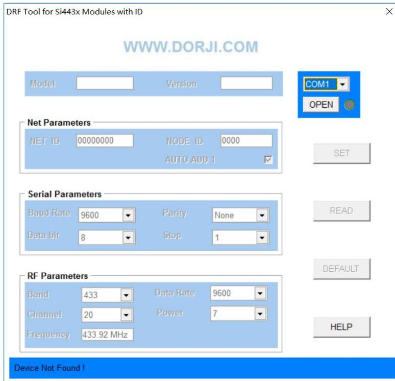
Figure 3: The Interface of inactivated DRF4432D20I Tool
