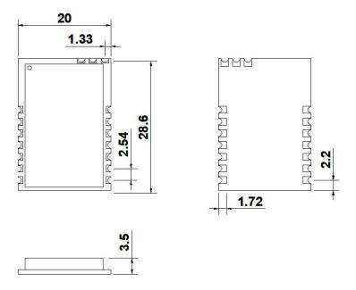
Figure 3: Mechanical Dimension
