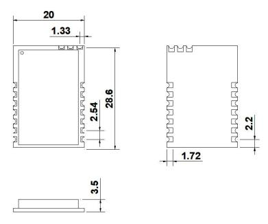
Figure 3: Mechanical Dimension
