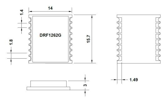
Figure 3: Mechanical Dimension
